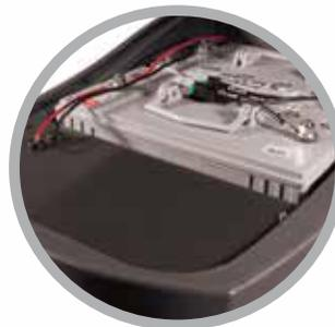
*Maintenance-free, gel batteries are standard*
