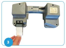
3. Please connect the 2 pin connector to the battery. It will only fit correctly in one direction. (C in figure 4)
